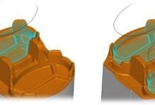
**NCG CAM** has an input tab available on all dialogs, once the passes have been made. This input tab, allows the user to change the input boundary or surfaces and re-calculate the passes.
