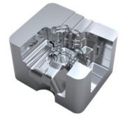
**NCG CAM**'s automatic roughing of surface data is suitable for all types of 2D or 3D forms, creating an optimised, smooth cutting motion suitable or high speed machining (HSM) while maintaining, part accuracy, cutting tool life and machine tool life. All cutters and tool-holders are collision protected to maximise efficiency and stock model visualisation of the machined part is available at every stage of the manufacturing process.
