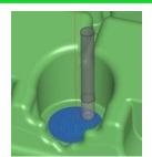
This creates an archimedean spiral toolpath from a given focal point, generating a constant contact as it machines within a given boundary. It is ideally suited for use on round shallow areas using contact angles between  $0^{\circ} - 30^{\circ}$ , in conjunction with the waterline machining for the more vertical faces  $30^{\circ} - 90^{\circ}$ .
