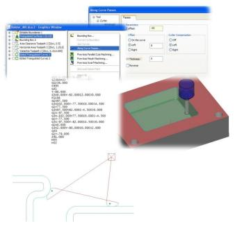
The optional pass overlap allows the cutter to overlap the starting position (closed profiles) to help reduce a 'tool line', giving a better surface finish.
