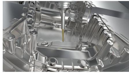
The better the surface finish means less hand polishing, which saves time and money, it also reduces any mis-match / flash caused by polishing rolling/belling corners.
